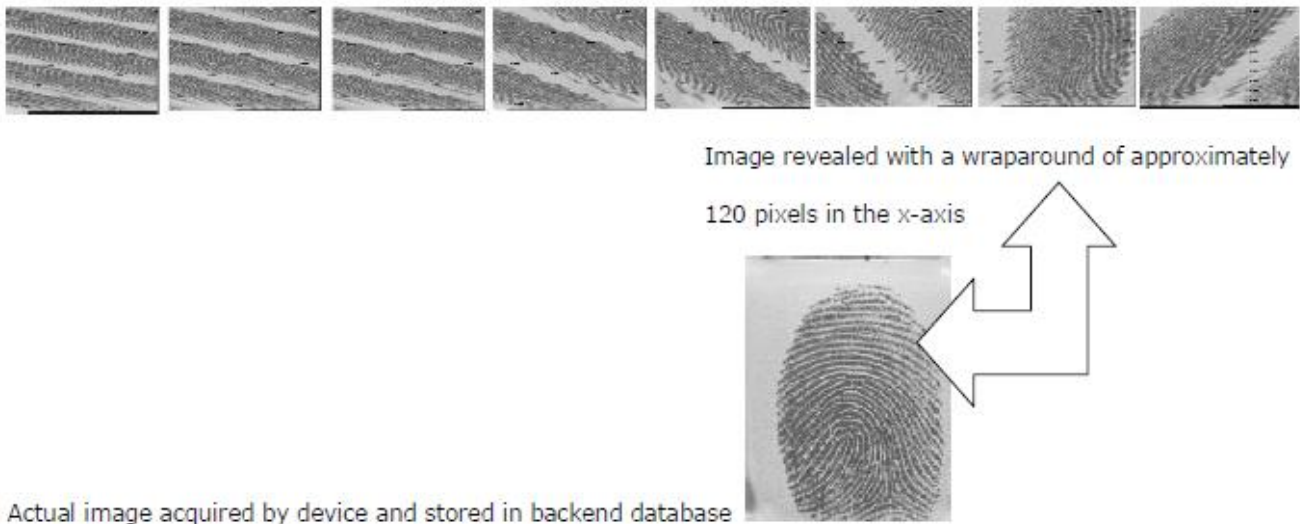
Figure 6. Successful identification of fingerprint image data from exchange between reader and management server.
